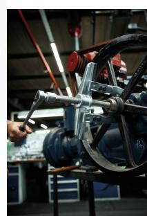
The adjustable puller arms make for universal use as both an external or internal puller possible.
