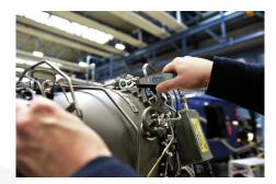
Displaying with acoustic, haptic and visual evaluation of the torque achieved.
