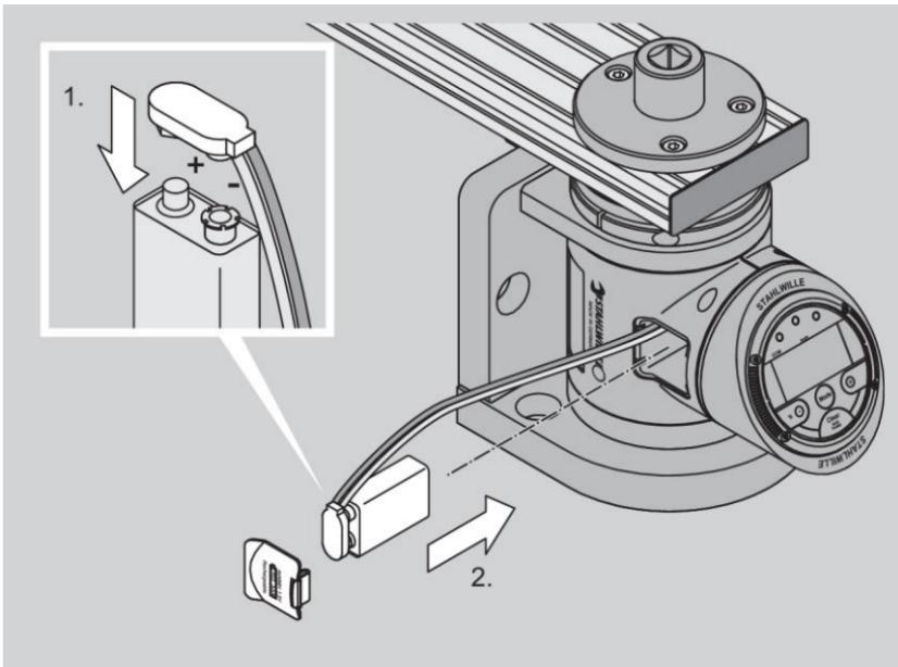
To use the adapter for four 1.5 V AAA batteries/rechargeable batteries, proceed as follows:
