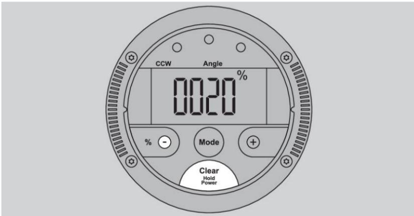
➤ Press the "–" button briefly until the desired tolerance value is displayed.
